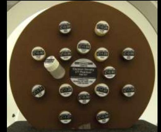
Measured by scanning a designed phantom, e.g. Catphan or RMI 467
