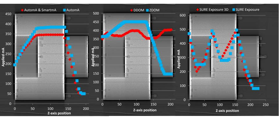
Demonstrates phantom (and couch) presents rotational variations in attenuation which are detected and accounted for by AEC systems
