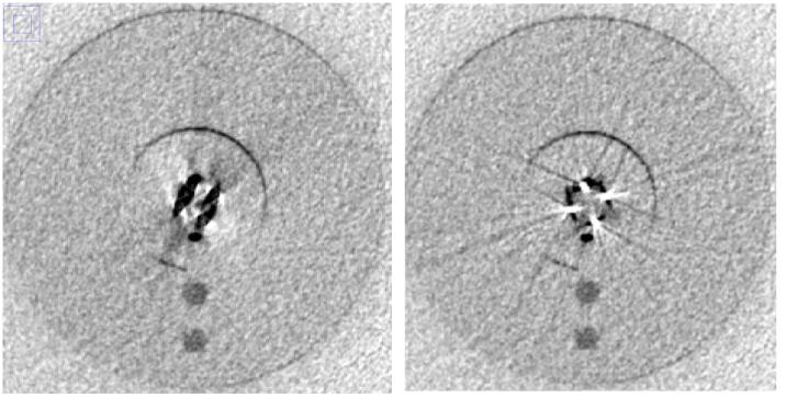
A 70keV reconstruction of a slice through a stent with (left) and without (right) MARS
