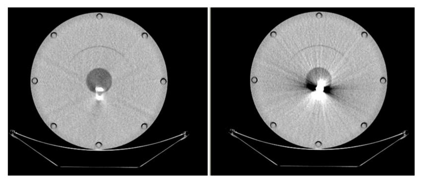
A 70keV reconstruction of a slice through a Hip Prosthesis with (left) and without (right) MARS
